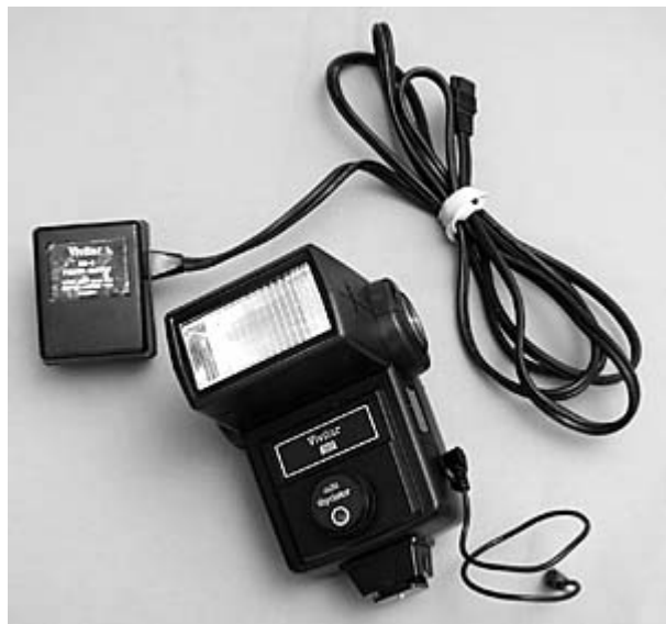
Figure 1. The Vivitar 283 electronic flash unit with SB-4 AC adapter and PC cord
