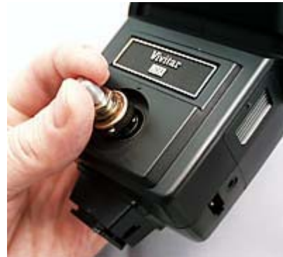
Figure 7. Variable resistor replacing auto thyristor module
