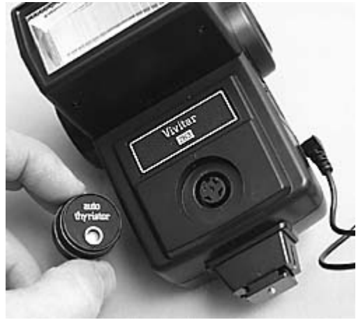
Figure 3. Vivitar 283 with auto thyristor module removed
