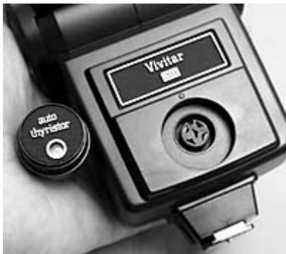
Figure 6. Auto thyristor module pulled out, revealing a socket of 5 holes
