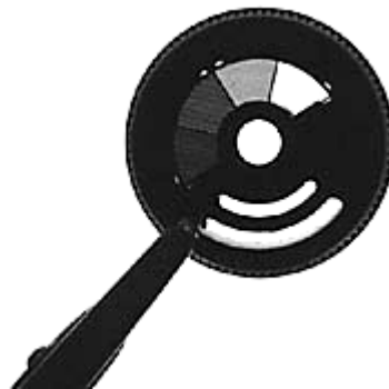
Figure 5. Neutral-density filters from an auto thyristor module
