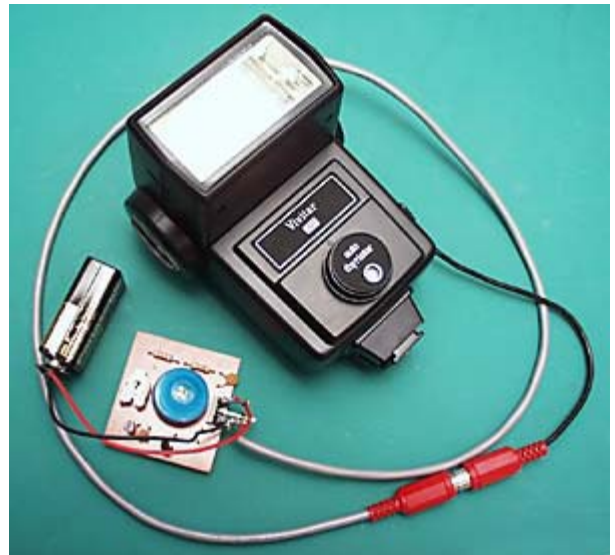
Figure 2. Sound trigger connected to a flash unit
